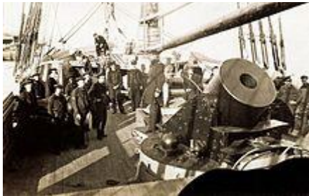
Main deck of Union Navy mortar schooner showing mounting of 13-inch seacoast mortar and crew.
